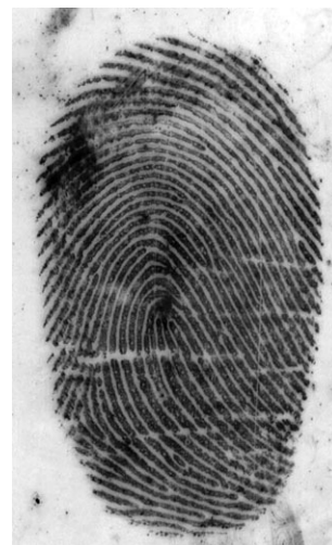
Fig. 21 Fingerprint on polypropylene stained with gold enhanced GNPs, and imaged with an office document scanner. Image courtesy of The School of Criminal Sciences, University of Lausanne, Switzerland.
