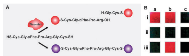
Fig. 6 Distance dependent detection of proteolytic enzymes. (A) In the absence of a substrate-specific protease (thrombin) GNPs are agglutinated by bivalent cysteine terminated peptides leading to a red-shift in their extinction spectrum. Cleavage of the peptide by thrombin prevents this. (B) Colours of GNP suspensions after exposure of the peptide substrate to the following cocktails of proteolytic enzymes: (ia) chymotrypsin, plasmin factor Xa and thrombin; (ib) chymotrypsin and thrombin; (ic) chymotrypsin, factor Xa and plasmin; (iia) factor Xa and chymotrypsin; (iib) chymotrypsin; (iic) factor Xa; (iiia) no enzymes; (iiib) thrombin; (iiic) plasmin; colours derived from ref. 44, Copyright The National Academy of Sciences of The United States of America.
